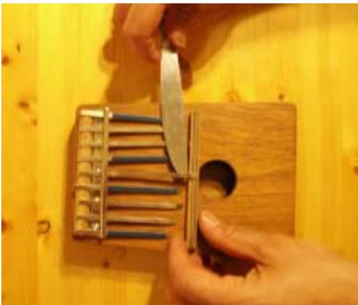
Step 9: reassemble the bridge from the wooden bar and the metal rod. Starting with the longest tines first, lift them up with a knife and ease them up onto the bridge. After each few tines is up on the bridge, nudge the bridge back towards the z-bracket so it is in position to get the next few tines up on the bridge.
