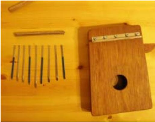
Step 6: rearrange the tines with the longest in the middle, next longest to the immediate left, third longest to the immediate right, etc, and imagine how it will look when it is all back together.
