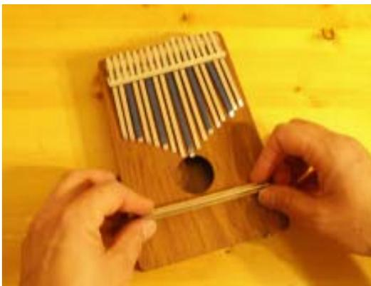
Step 2: Admire your work. The bridge has a metal rod on a wood bar, and they are held in place only by the tension of the tines pushing down. Likewise, the wood back stop at the head of the tines is also held in place by the tension of the tines. Now, any of these pieces could just fall away, but keep everything orderly for the following steps.
