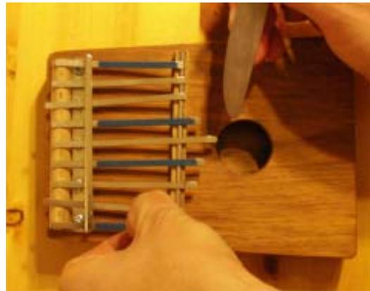
Step 10: push the bridge back up into place using that butter knife again. This step requires some strength in your hands and fingers.
